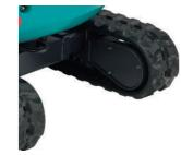
For added protection, Kubota has enclosed the travel motor hoses within the track frame, resulting in reduced repair costs and increased durability.
