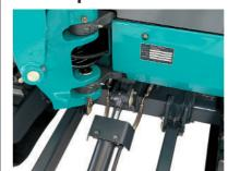
Two-piece hose connections for the dozer simplify hose replacement, reduce downtime.
